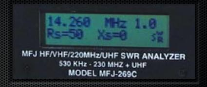
It's always preferable to measure SWR rather than resonance or impedance magnitude (Z) as the standard for adjusting your antenna.
