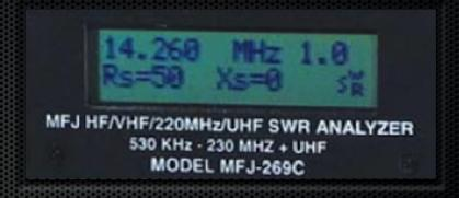
If your antenna doesn't happen to present a 50-ohm load at resonance, there will still be resistive mismatch (and SWR) in the system. In fact, slightly lower SWR may actually occur on some other frequency. By the same token, if you adjust your antenna for an Impedance reading of 50 ohms, it may have a substantial reactive component (for example R = 46, X = 17) that would elevate SWR and shift the minimum-SWR point to a different frequency.
