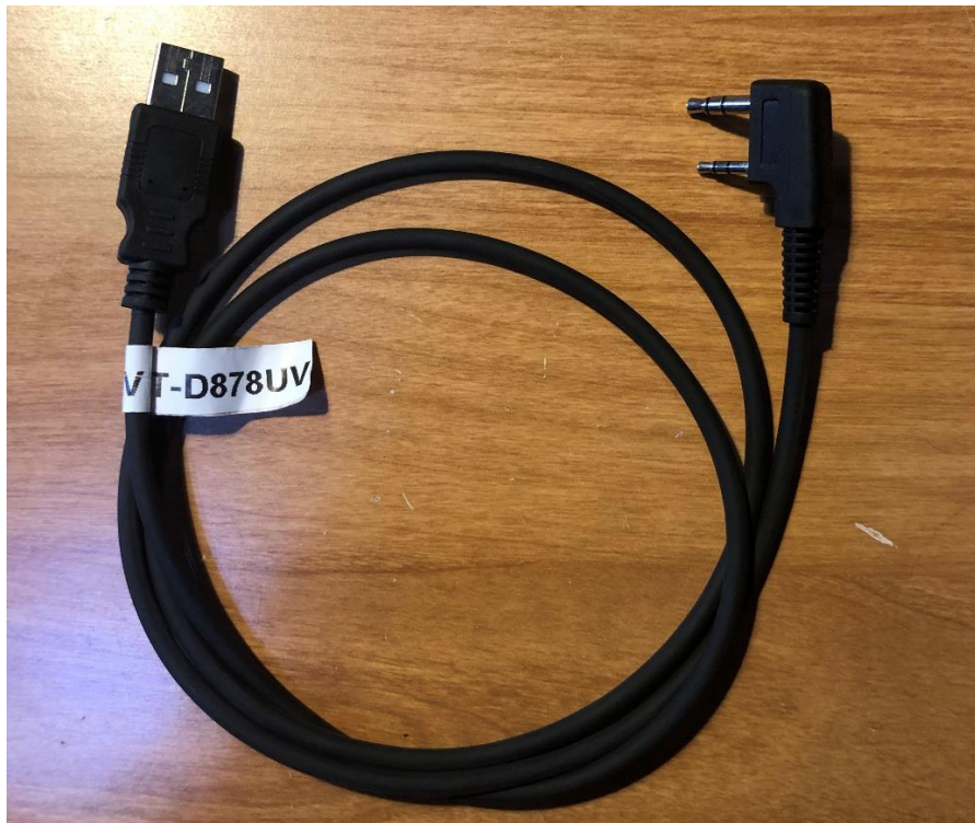
Figure 1. AT-D878UV programming cable, which I labeled to distinguish it from other cables.
